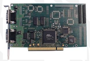
Hardware configuration via PCI software services (plug-and-play). A DPRAM interface for host interfacing is available. The customer can use LevelX (DLL) for the easy programming of own complex applications. With the *PCI-IntelliCAN* a powerful hardware solution is available for a CAN interface card.
