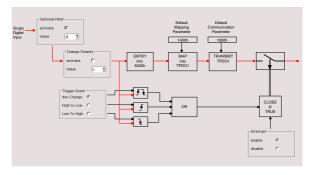
port and provides functions for realizing I/O devices that conform to the device profile CiA 401. The implemented functions realize the functionality as specified in the standard, i.e. logic operations, polarity switching, filter mechanisms, limit monitoring and others. The developer has to provide functions to access the hardware, ie. reading inputs, writing outputs.
