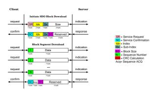
SDO transfers are based on the client-server model with a handshake after each transfer. For a larger block of data this will take a large amount of time. Therefore a new SDO mode has been defined in CiA 301 V4.x. It is called SDO block transfer. Using the block transfer a sequence of blocks can be transmitted without a large overhead. Each block is a sequence of up to 127 segments (e.g. CAN telegrams)
