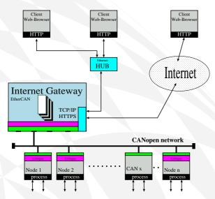
Sending CAN message via the CAN server is possible, too. In the easiest case the server is used as a CAN analyzer via the Ethernet. The CAN Analyzer CAN-RE*port* can be used for this.
