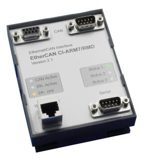
The *EtherCAN* Gateway combines the decentral CAN and CANopen networks with the classical Ethernet network. To communicate via Ethernet the TCP/IP protocol is used, while on the CAN bus the communication is realized by CANopen, DeviceNet or another user-specific protocol.
