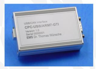
The CAN interface supports 11 and 29 bit CAN identifiers. The on-board 32-bit ARM micro controller system Philips LPC2119, with 128 KByte FLASH and 16 KByte RAM, is capable to control transmission and reception tasks with the highest efficiency possible. *CPC-USB* is powered by the USB bus, no additional power supply is required. Development kits for developing applications using *CPC-USB* are available for the operating systems Windows<sup>TM</sup> and LINUX<sup>TM</sup>.
