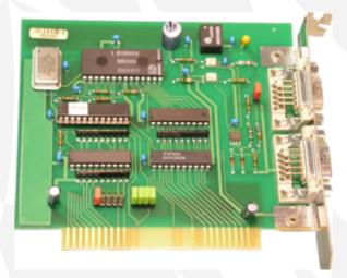
The component is suitable for all kind of applications, where the main processor provides sufficient computation power to serve the Basic-CAN/PeliCAN interface in an application specific manner.
