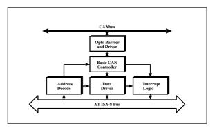
The interface to the CAN bus is provided by connectors compatible with ISO/DIS 11898 and CiA recommendations.
