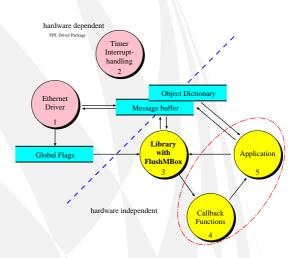
The POWERLINK *Library* consists of a hardware independent and a hardware dependent part that communicate with message queues. The hardware dependent part consists of controlling software for the Ethernet MAC controller and timer functions.
