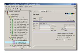
The graphical POWERLINK *Design Tool* is available for the creation of the object directory, the electronic data sheet (EDS file in XML format) and for the documentation of the device in HTML or text format.
